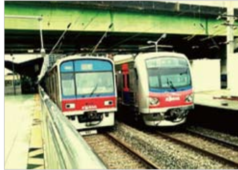
Figure 8.10. Driverless car in Shinbundang line
