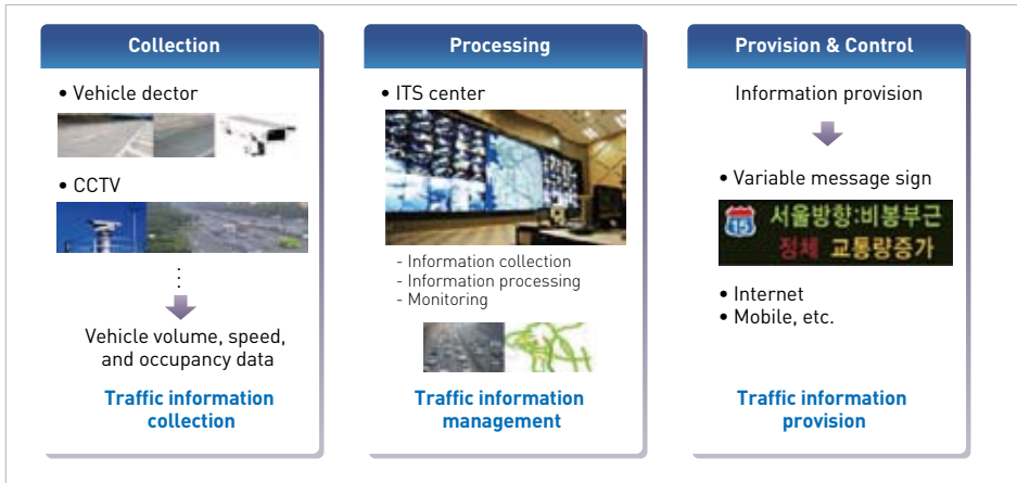
Figure 9.19. Process of the traffic information service (collection, processing, provision)
